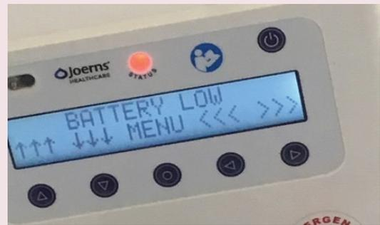
**LOW BATTERY** - For inline charge systems the lift unit will charge anytime the hoist is not in use. When the batteries charge level reaches a low condition, the charge / status indicator will flash red and, in ambient light conditions, this will be accompanied by an audible beep each time an operating control is depressed. In low light conditions, only the charge / status indicator will flash red.
